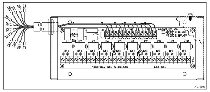
Figure 6-32 Ten-Relay Dry Contact Kit
